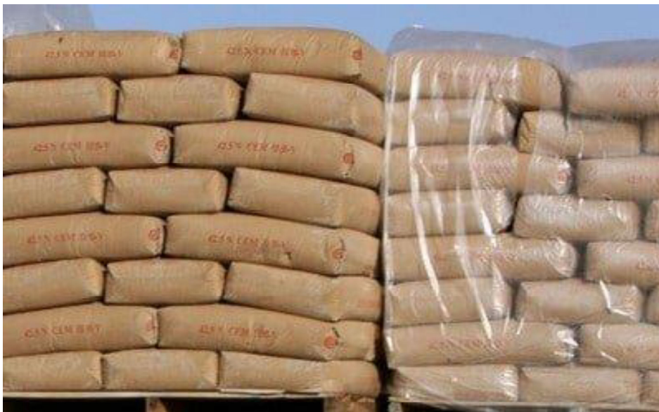
Cement bags are arranged alternate length and crosswise for 8 or more row stacking
