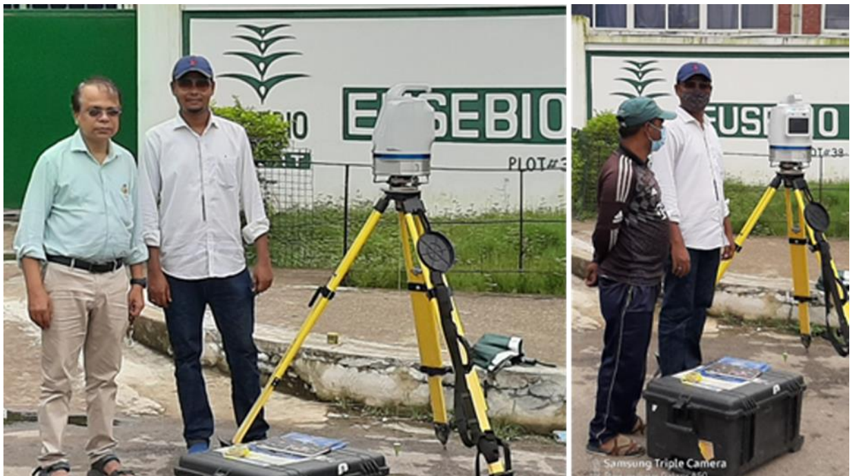
Survey of Land and Structure point cloud (x,y,z data) collection
